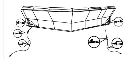
Safety Note: Transformer and cables are not to be placed under or within the recliner structure.
