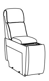
STEP 3: Install back 6 onto seat 7.
